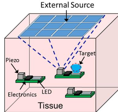
Fig. 1. Futuristic conceptual representation of a multi-node ultrasonically powered optogenetic system with beam-forming capability. The figure is not to scale.
