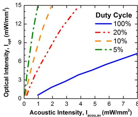
Fig. 3. The achieved optical intensity as a function of the average acoustic intensity, for different duty cycles.
