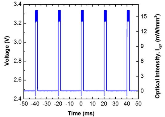
Fig. 4. Output voltage of the TIA and optical intensity of modulated light pulses with 50 Hz frequency and 2 ms pulse-width. Dark blue areas are 955 kHz ripple from capacitive feedthrough - this has no impact on the optical measurements.
