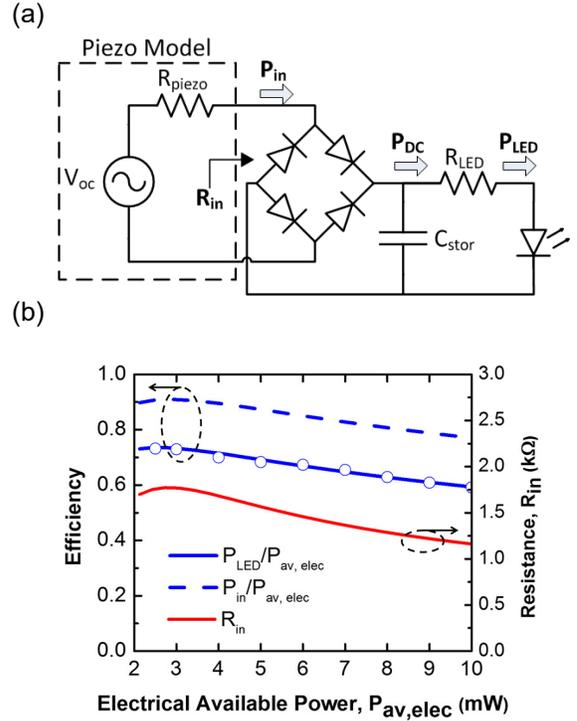
Fig. 2. (a) Schematic of the implant used in this demonstration. (b) Measured (circles) and simulated  $P_{LED}/P_{av,elec}$ , simulated  $P_{in}/P_{av,elec}$ , and simulated  $R_{in}$  as a function of  $P_{av,elec}$ .
